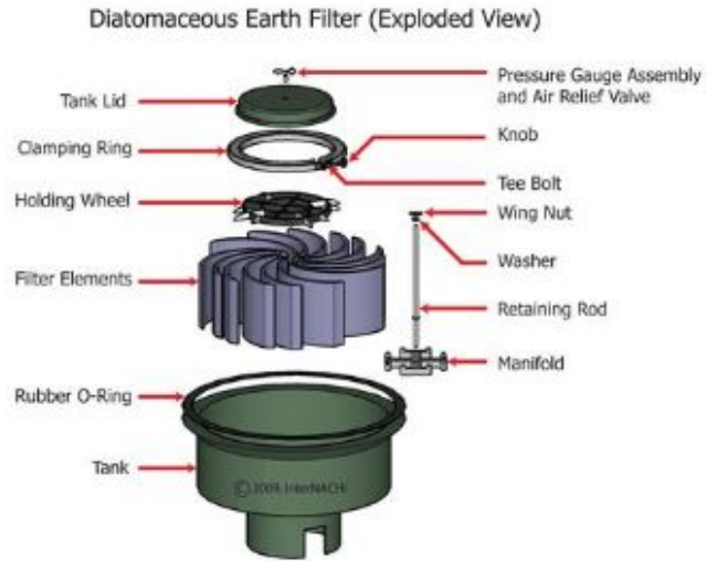
Internal View of a DE Filter
